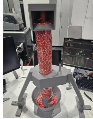
Figure 4: Experimental demonstration of the VMDC, showing vertical conveyance.
