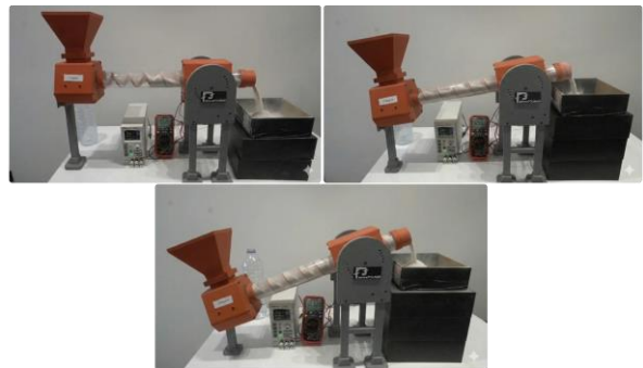
Figure 2: Experimental setup of the MDC prototype demonstrating material conveyance tests conducted at distinct orientations 0° (top left), 10° (top right), and 20° (bottom center).
